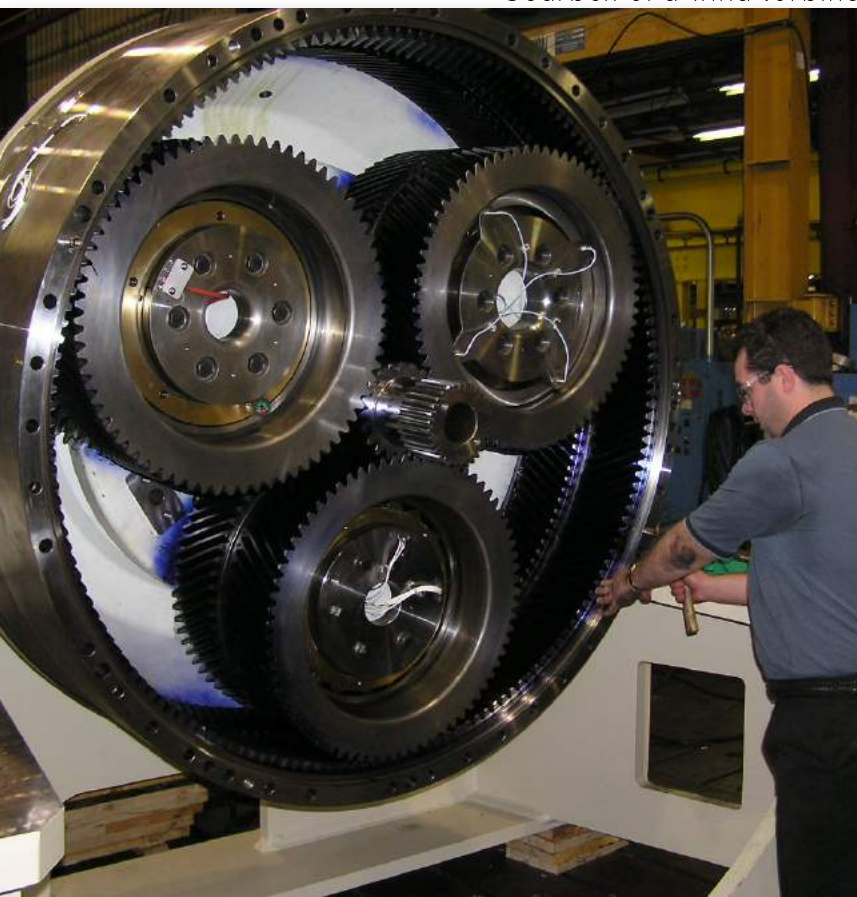
Gearbox of a wind turbine
